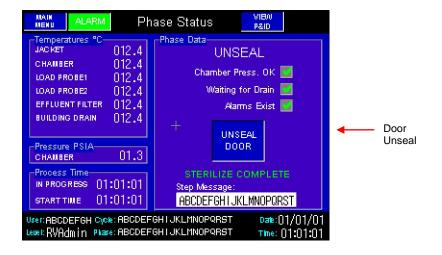
The door will then automatically unseal just as it did above. After the door is unsealed, the Start Cycle screen will appear displaying a CYCLE COMPLETE button and an audible tone will sound.
