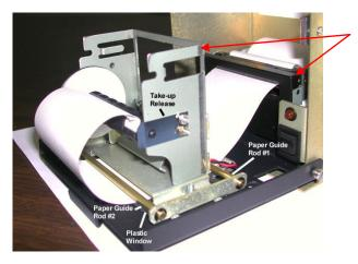
Printer Ribbon – grab both sides and pull to remove
