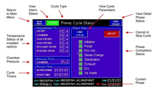
The Phase Data box provides a list of the phases required for the type of cycle you are running. A green  $\square$  indicates the phase has been completed, a yellow  $\boxtimes$  in check box indicates the phase is not completed. The phase currently running is displayed in the center bottom of the status bar.
