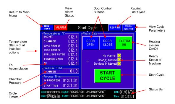
To start a cycle, the system must be in the ready state. This means there can be no active alarms, the door(s) are closed, and the system is in automatic mode. The Ready Status is displayed above by the 3 green  $\checkmark$ , if the system was not ready, one or more of the check marks would be a yellow  $\Join$ .
