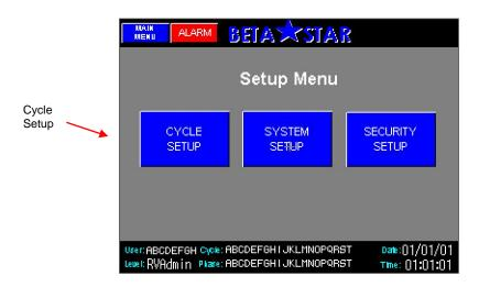
From the Setup Menu screen push the CYCLE SETUP button, this will bring up the Select Cycle to Setup screen shown below.
