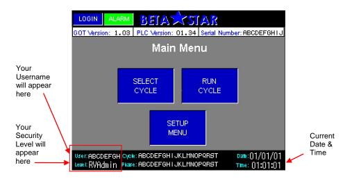
From any screen that contains the status bar, you can login or logout by pressing the area of the status bar that contains the User name and Security Level. See red box above.
