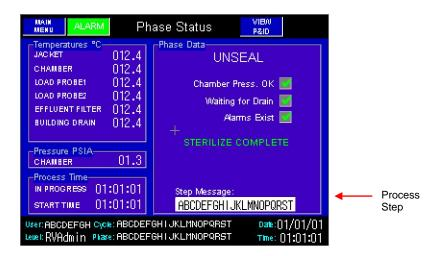
On a non-interlocked or multi-flow double door unit, the screen will look like the one below. This screen will show up on the HMI at both doors allowing the operator to unseal either end. To unseal the door the operator must press the UNSEAL DOOR button on the HMI at the door they wish to unseal.
