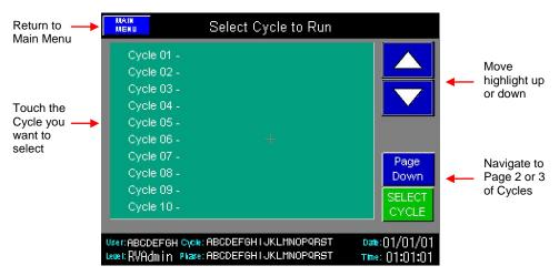
To select a cycle, touch the cycle you want to select, or use the arrow buttons to move the screen highlight to the cycle you would like to select, then press the SELECT CYCLE button. You can Page Down for more options, the system holds a total of 30 cycles.
