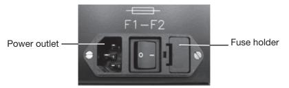
This unit is protected by two fuses (5 x 20 mm, 2A Slo-Blo). The fuses are located in the left side rear of the universal hood, in a fuse holder housed in the power entry module.
